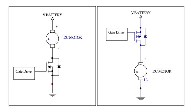
Figure 1: Single-Ended High-Side Drive Schematic Detail
