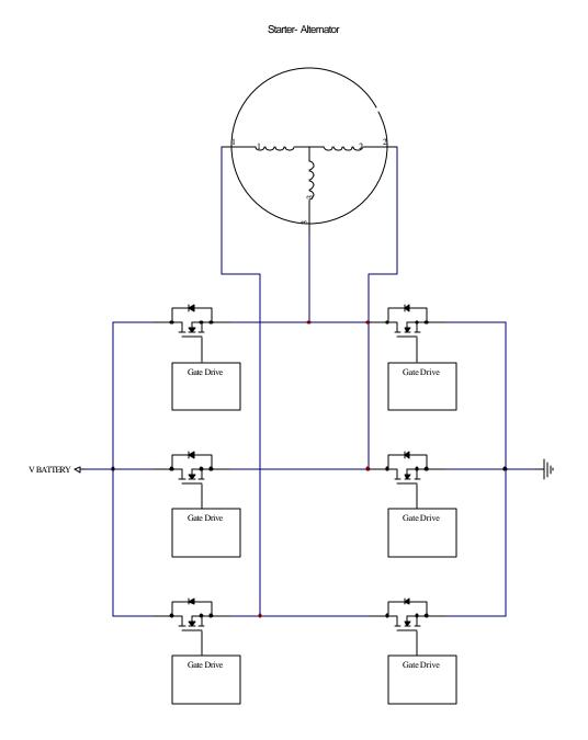
Figure 4: Integrated Starter and Alternator in a 3-Phase Bridge Configuration
