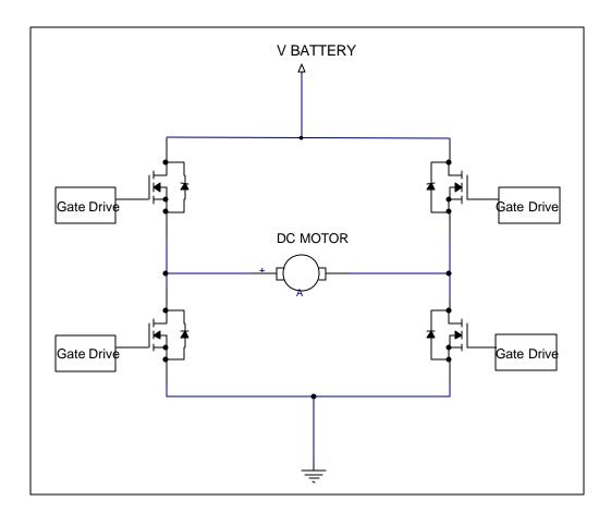
Figure 3: Full Bridge Configuration Schematic Detail
